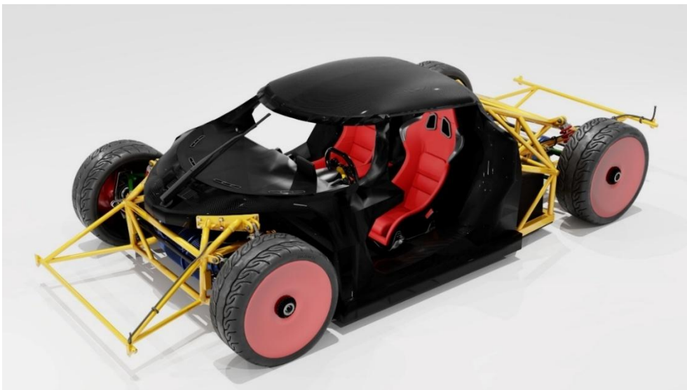
Figure 2 – Dubina Evo with the front-mounted powertrain.
