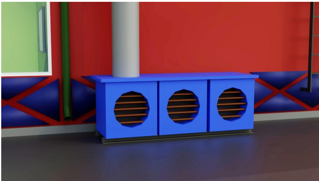
Figure 15 – Heat exchangers of the climate control system
